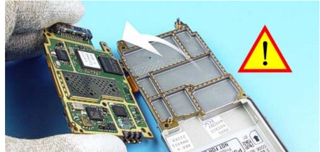
46.) Turn the Engine Module. Take care of the RF Gasket .
