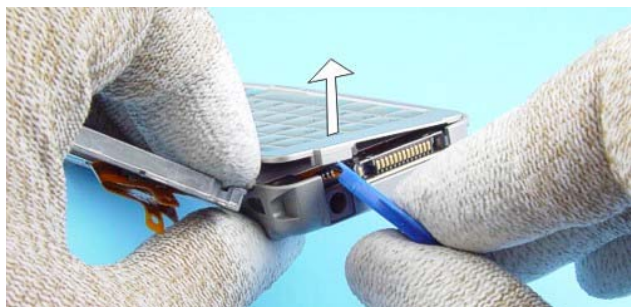
24.) Place the SRT-6 between Qwerty Keypad and the DC-Jack and lift the Qwerty Keypad carefully.
