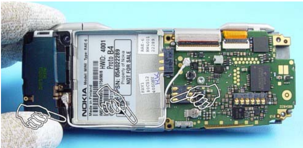
34.) Note the placement of the RF Coax Cable before continuing the disassembly.
