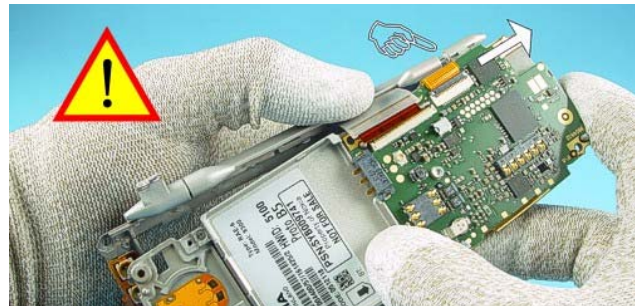
42.) Separate the 1CP QWERTY Flex Module from Chassis .
