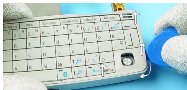
26.) Unlock the hooks along the edge of the Qwerty Keypad as shown.
