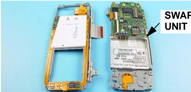
43.). Note! Do not follow the next steps (44-47) in case you have to swap the 1CP QWERTY Flex Module . Look forward to chapter 10 => SWAP UNIT Assembly (Editional instructions) .
