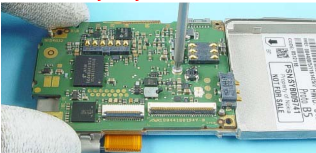
Always use new screw when re-assembling! For assembly use a Torx Plus® size 6 driver with a torque setting of 25Ncm.
