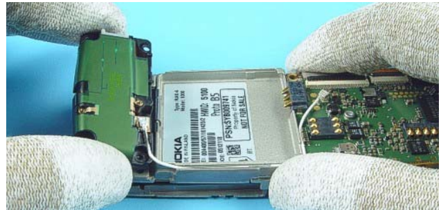
35.) First remove the Antenna Assy . Do Not open the Antenna RF connector!
