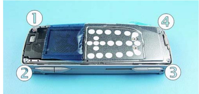
8.) Unscrew the four, Torx Plus® size 6 screws in the shown order. Always use new screws when re-assembling! For assembly, reverse the order and use a Torx Plus® size 6 driver with a torque setting of 25Ncm.
