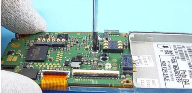
45.) Unscrew the Torx Plus® size 6 screw.
